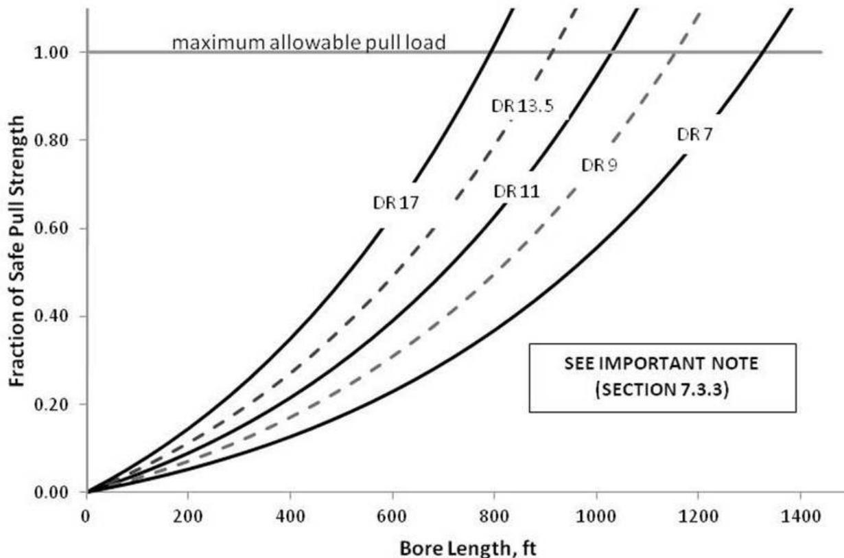
**Figure 9 Predicted Mini-HDD Pull Load vs. Safe Pull Tension, HDPE (PE4710) Pipe Nominally Straight Path, 2-inch Drill Rods**
