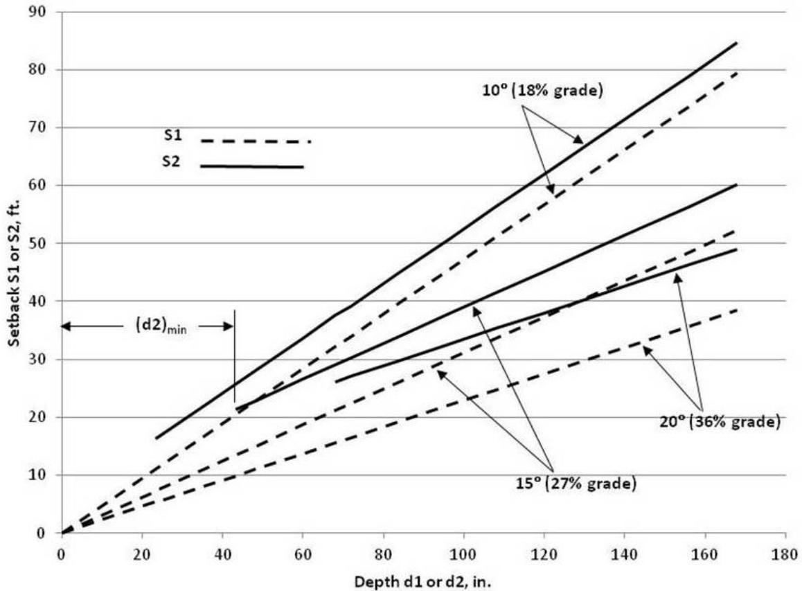
**Figure 13 Drill Rig Setback Distance**
