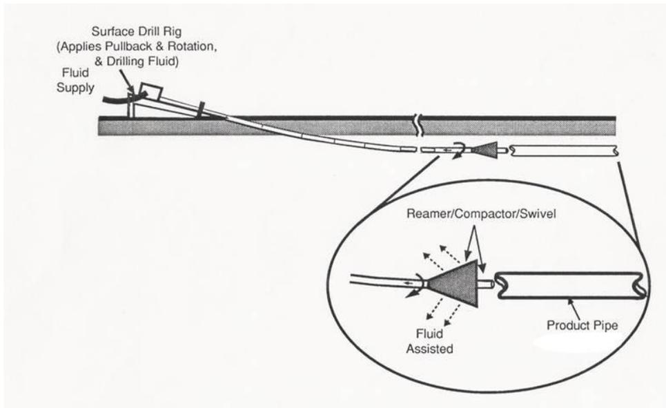
**Figure 2 Typical Mini-HDD Back-Reaming and Pipe Pullback Process**
