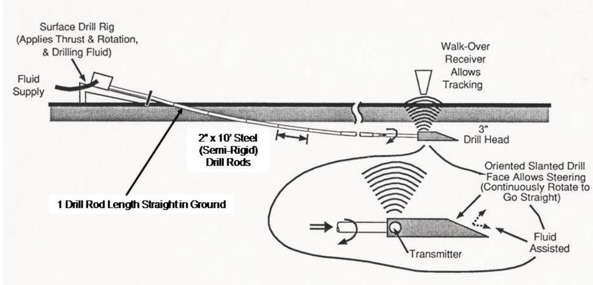
**Figure 1 Typical Mini-HDD Equipment and Pilot Boring Process**
