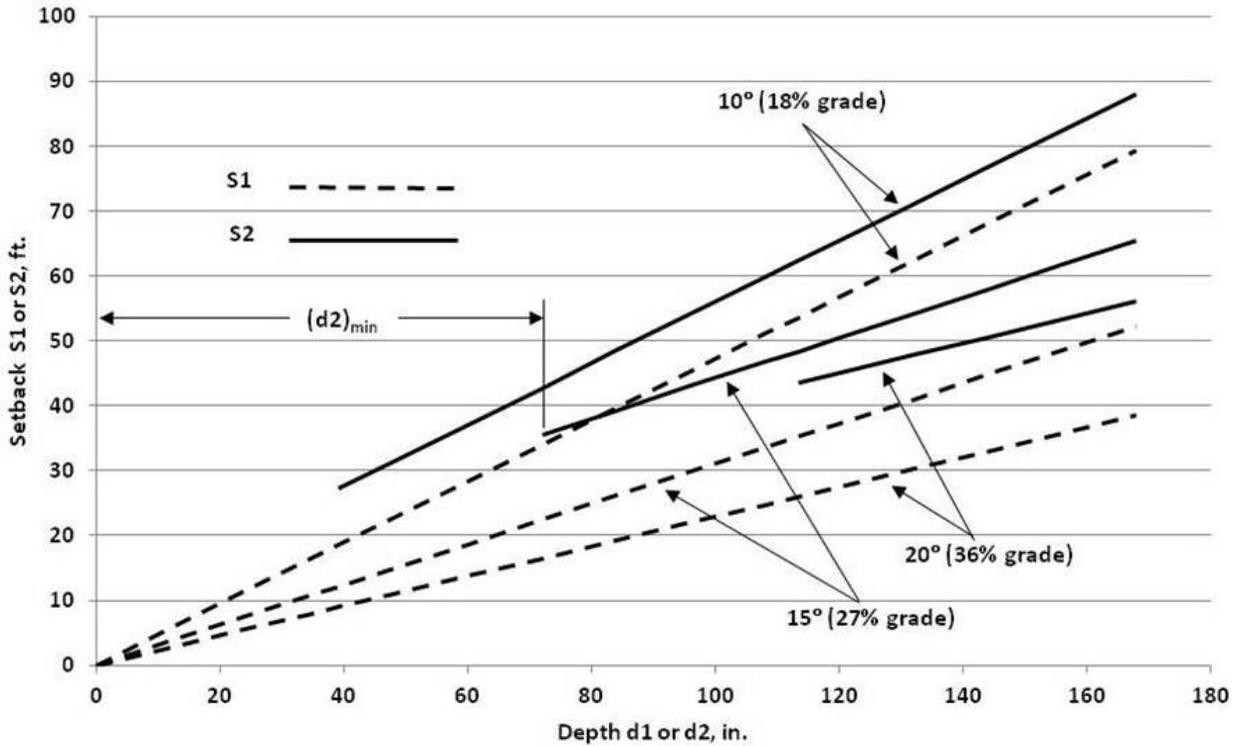
**Figure 14 Drill Rig Setback Distance**
