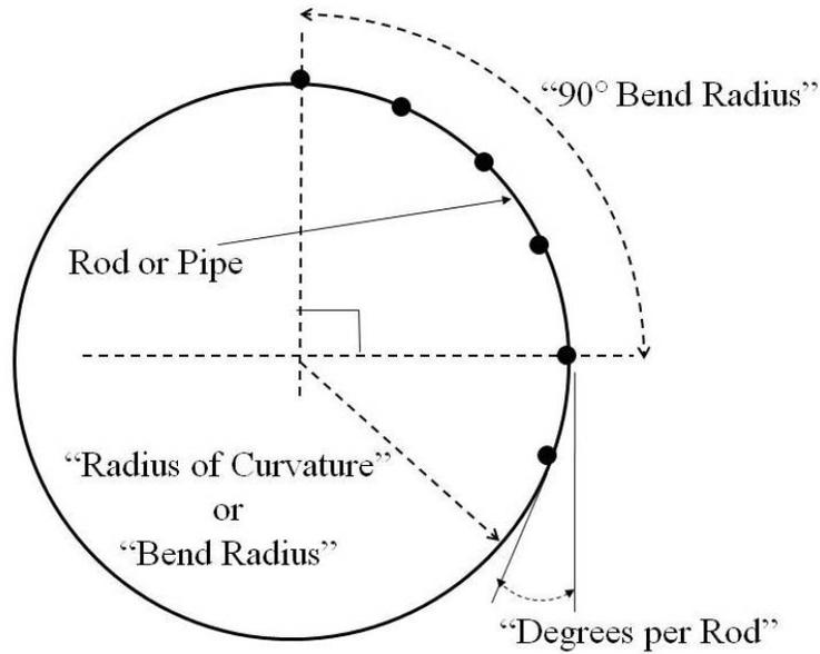
**Figure 3 Rod or Pipe Curvature Terminology**
