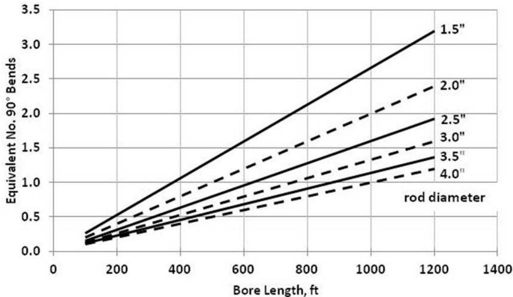
**Figure 8 Unplanned Curvature,  $n_2$**
